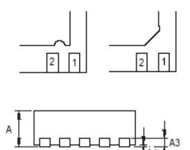
DETAIL A Pin#1 ID and TIE Bar Mark Options Note: The configuration of Pin #1 identifier is optional, but must be located within the zone indicated.
